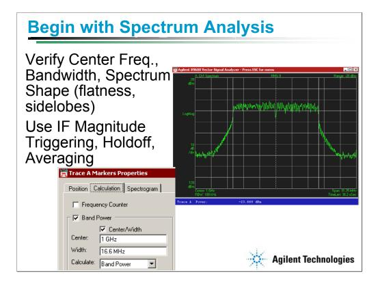
Before attempting more advanced tests such as burst analysis or digital demodulation, it is always advisable to confirm basic signal parameters such as center frequency, bandwidth, and spectral shape.
