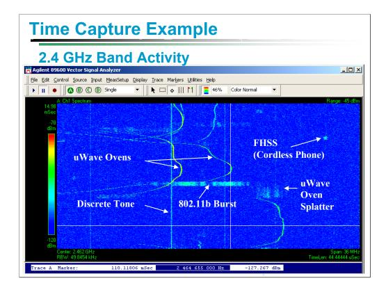
This is a spectrogram of a portion of a time capture from the 2.4 GHz band where 802.11b and 802.11g operate. It shows the challenges facing designers of this equipment. Many different sources of interference may be present at the same time, and need to be understood and dealt with.
