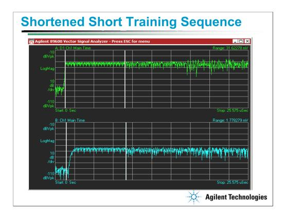
This is an example of a real signal (bottom trace), with a problem in the short training sequence. The sequence is truncated, as shown by the 8 us gate markers and the reference signal at the top.
