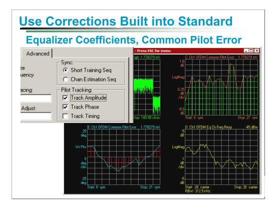
In OFDM, demodulation is performed relative to the pilot signals, after correction by the adaptive equalizer.
