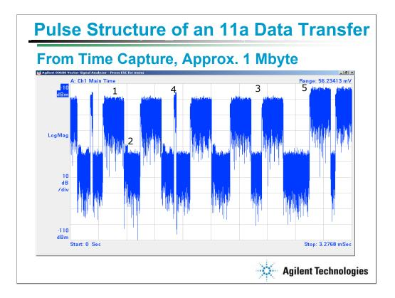
Using the recorded waveform, it would be simple to zoom in to examine every part of the burst in detail.
