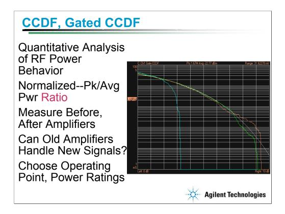
OFDM signals make particularly high demands of power amplifiers. Their peak/average power ratios are much higher than CCK signals and many other types of digitally modulated signals.
