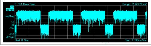
Time capture is a particularly powerful function for measurements such as these. It ensures that no information is missed during the capture, and that all data in the measured bandwidth is available for any type of post-acquisition analysis.
