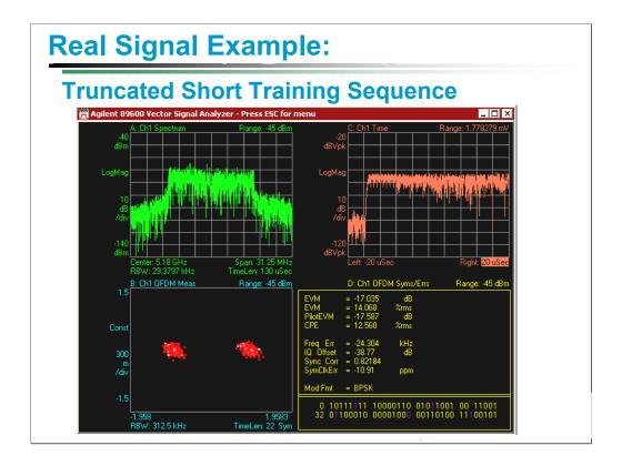
This slide shows demodulation results from a real signal, on a system that is working. This is the signal with a truncated short training sequence as shown on a previous slide.
