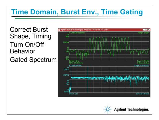
Measurement of burst shape and timing parameters is especially important in signals such as these, as errors here may create interoperability or compatibility problems.
