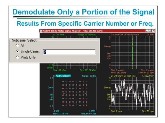
In an OFDM signal it can be useful to look at a limited set of demodulation results. In this case demodulation, and the errors and symbols to be measured, are limited to a single carrier number. The data from this carrier only is shown in the constellation in the lower left.
