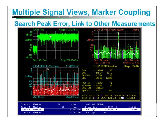
One of the most powerful diagnostic tools is the coupling of results from different simultaneous measurements.
