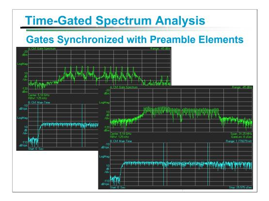
Two gated spectrum measurements are shown, both of the OFDM signal in the previous slide.
