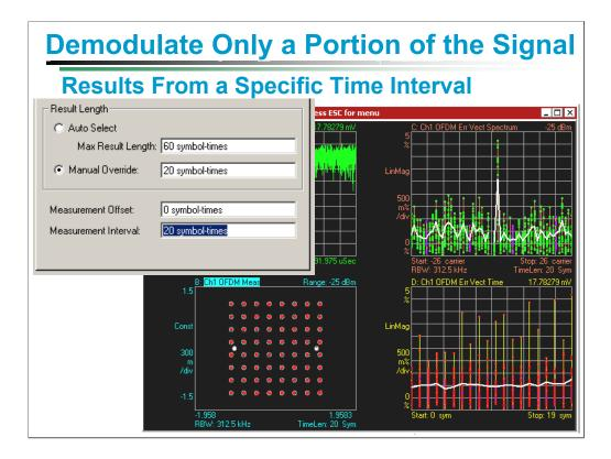
Demodulation results can be limited to a specific time period, to investigate impulsive errors or interference, for example.
